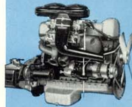
3-liter 6-cylinder high-powered engine 136 HP at 4,500 r.p.m. overhead camshaft, 2 multi-stage carburettors with automatic choke.
